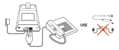
$\label{lower} \textbf{IMPORTANT} \ \textit{Use configuration A} \ \textit{on the bottom of the base, which works for most phones including Cisco phones.}$
