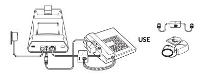
**IMPORTANT** *Cisco* phones use configuration **D** on the bottom of the base. Most other phones use default configuration **A**.
